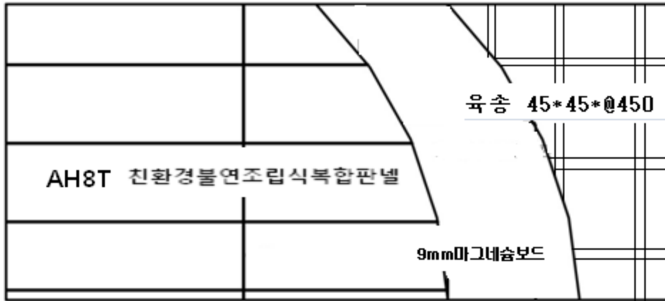
Plane figure of the installed Hi-Top fire resistant Panel (AH 8TS)
